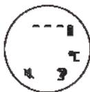
With the device switched on, press and hold the ON/MEM button for 3 seconds. The silent mode symbol
