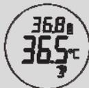
This function is valid in ear and temple measurement mode. For every new temperature measurement, the result from the previous measurement will be shown for comparison at the top of the LCD display.
