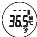
With the device switched on, repeatedly press the ON/MEM button to display up to 25 previous measurements. The memory is represented by the
